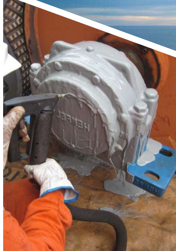
MINING - PROTECTION OF BEARING HOUSING Lifespan increases several times on bearings subject to contamination by particulates.
