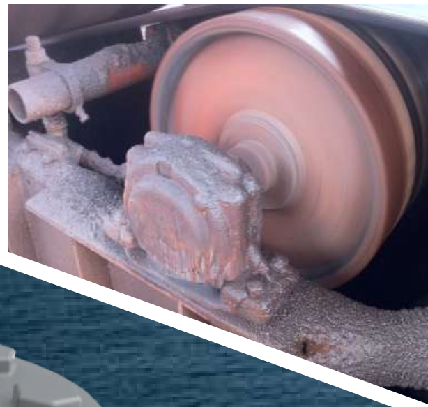
MINING - PROTECTION OF BEARING HOUSING Lifespan increases several times on bearings subject to contamination by particulates.
